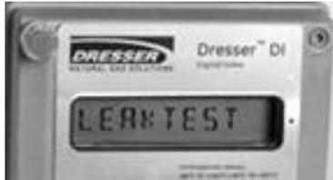
Figure 7: Leak Test (LEAKTEST) LCD screen
