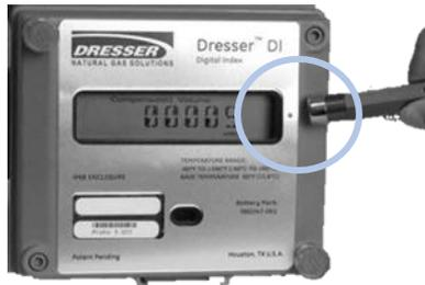
**Figure 2: Magnet used to change screens**
