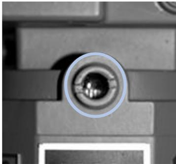
**Figure 3:** Flow Indicator location under cover in meter
