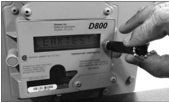
Figure 5.7 - Scroll to LEAKTEST screen.
