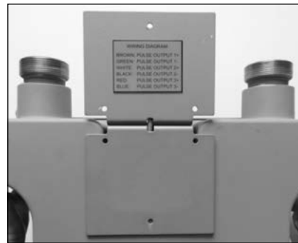
Figure 7.10 -Properly positioned mounting bracket
