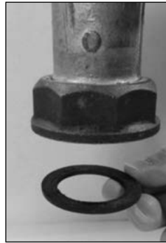
Figure 5.1 - Proper installation of washer into swivel
