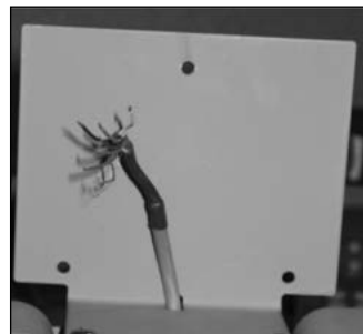
Figure 7.11 -Pull cable through the center hole
